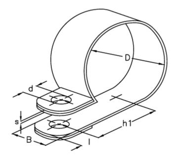
$\begin{array}{ll} d & = 8.4 \\ \text{Diameter D} = 10 \\ \text{h1} & = 17.5 \\ \text{I} & = 8.5 \\ \text{s} & = 0.8 \\ \text{Width B} & = 20 \\ \end{array}$
